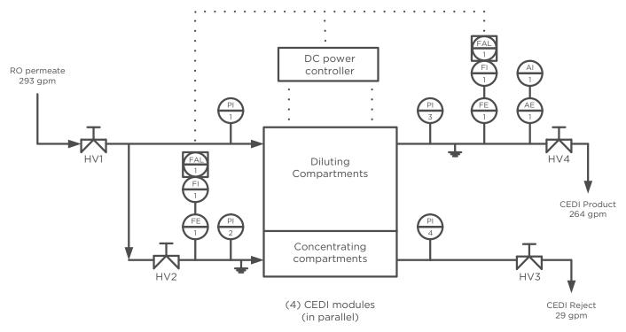
Figure 3 P&ID of 264 gpm (60 m<sup>3</sup>/h) CEDI system
